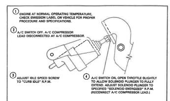
A/C IDLE SPEED ADJUSTMENT W/SOLENOID
