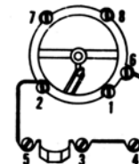
AIR HORN TIGHTENING SEQUENCE
