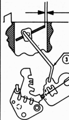
CHOKE ROD ADJUSTMENT Fig.15
