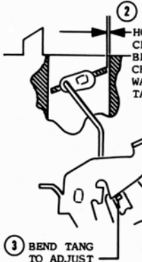
CHOKE UNLOADER ADJUSTMENT Fig.17
